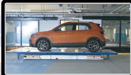
AGV transports the pallet with the car to a vacant parking system
